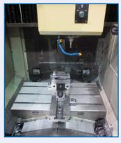
**HITACHI SEIKI** VM40II, Seicos CNC control, travels: X-22.05", Y-16.14", Z-16.14", table size 16" x 30", distance from spindle to table 5.9"-22.05", 8,000 RPM, 40 taper, 20 internal sidemount ATC, tapping, flood coolant, chip auger, sn 42251
