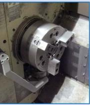
HITACHI SEIKI HT23SII, 10" 3 JAW CHUCK HITACHI CNC CONTROL, 10 STATION TURRET, TAILSTOCK, TOOL PRE SETTER, 3,600 RPM, SN HTS 2746HL
